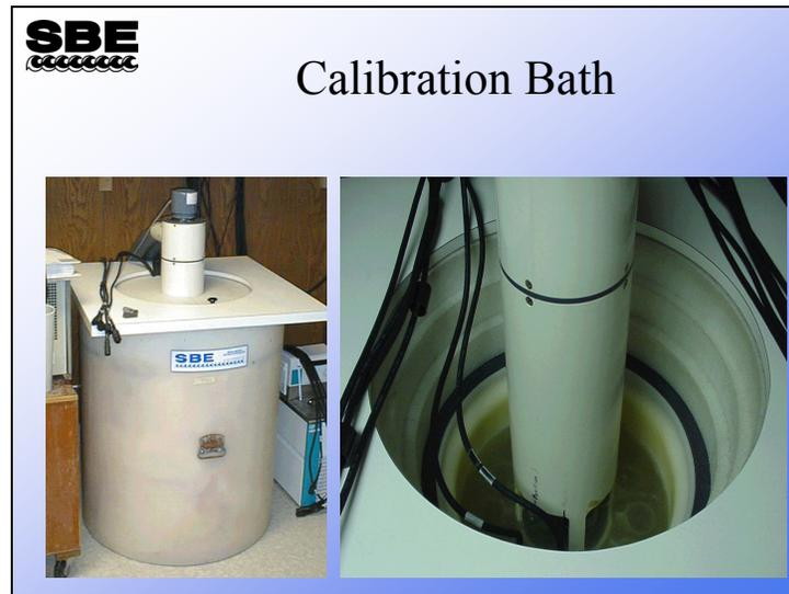
This bath design is common to all of Sea-Bird's calibration activities. They are highly insulated and well stirred, and they typically hold temperature to better than 0.0005 °C.
