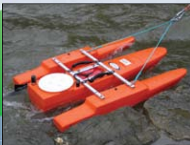
Teledyne RDI's Rio Grande ADCP allows you to collect real-time discharge measurements from any moving platform—from small tethered boats to inland survey vessels.
