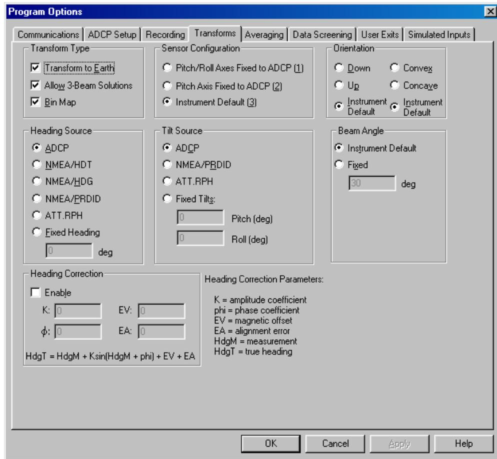
Click the **Transforms** tab and verify that the **Transform Type**, **Sensor Configuration**, **Orientation**, **Heading Source**, **Tilt Source**, **Beam Angle**, and **Heading Correction** are set to your input.
