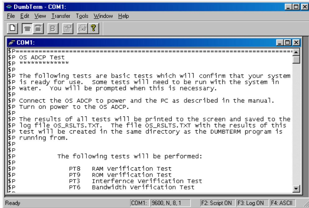
**Step 2.** Run *DumbTerm* to verify the ADCP is functioning properly. Select a script file from the table below. The results of the tests will be saved to an ASCII text log file.
