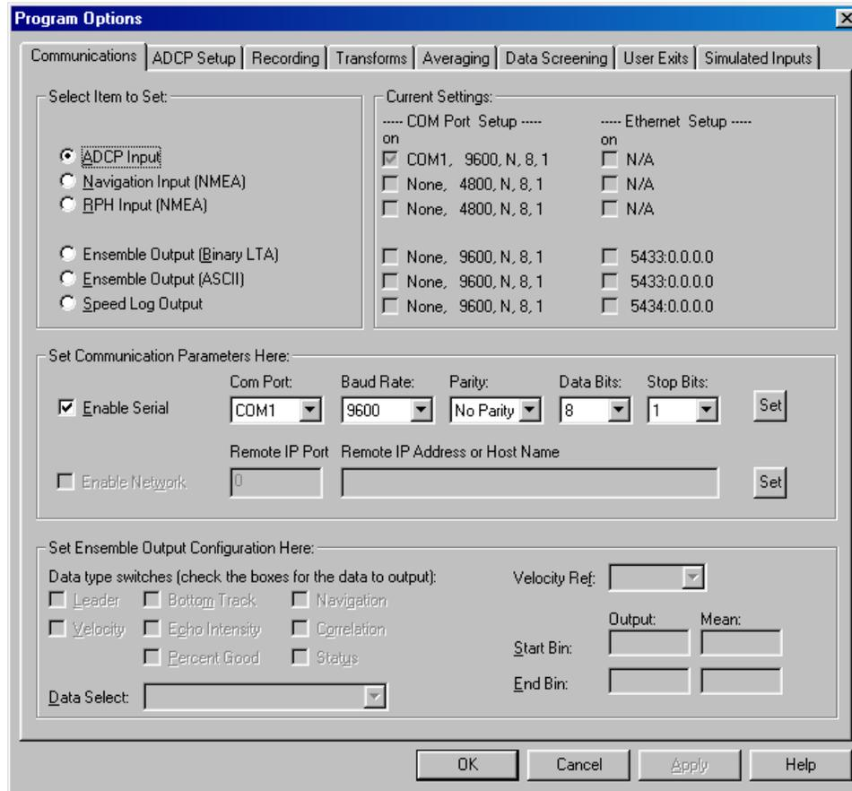
Click the **Communications** tab and set the communications settings with the ADCP and NMEA ports.
