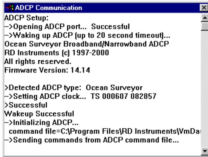
**Step 6.** On the **Control** menu, click **Go** to begin collecting data. The ADCP Communication window will open and show the commands from the command file being sent to the ADCP and the ADCP's response. Once all of the commands have been sent, the window will close automatically. See "[VmDas ADCP Initialization](#)," page 31 for details on how the ADCP commands are generated and sent to the ADCP.
