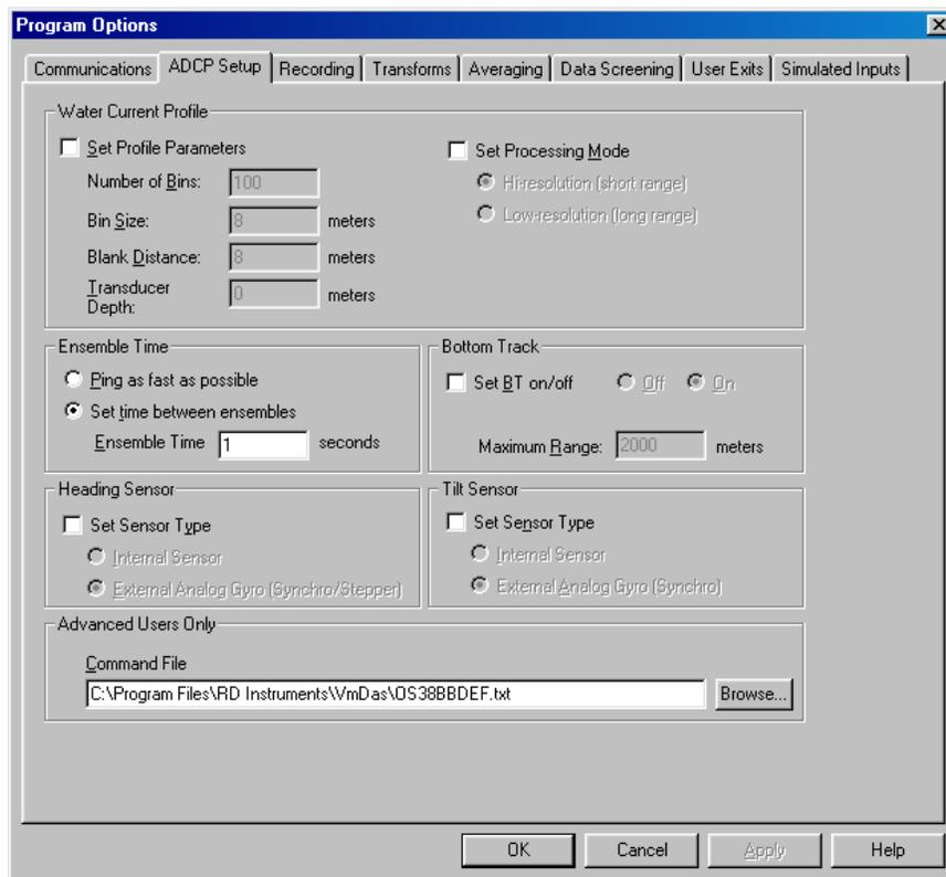
**Step 4.** On the **Options** menu, click **Edit Data Options**. Click the **ADCP Setup** tab. Make sure that *all* boxes in the **ADCP Setup** tab are *unchecked*. Set the **Ensemble Time** to the value shown in [Table 1](#).
