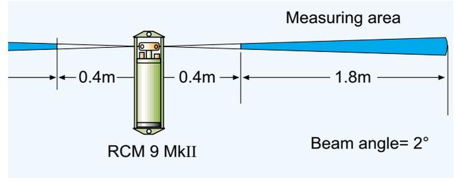
The instrument can operate continuously or in eight intervals from 1 to 120 minutes. At 60-minute recording interval the operating time is more than two years.
