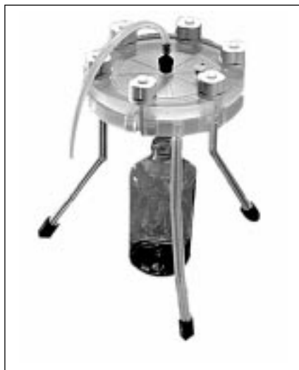
Figure 2-13. Nonmetallic backflushing plate-filter assembly for 142-millimeter diameter filter media. (Illustration reproduced with permission of Gelman Sciences.)
