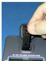
Photo 2. Placing the adjustable secondary standard in the AquaFluor™
