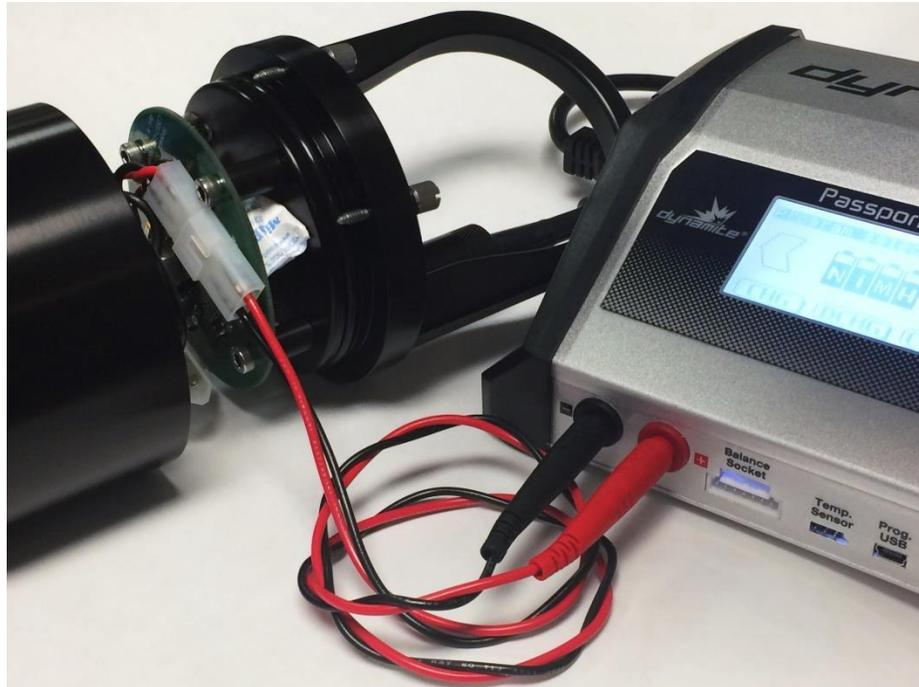
On the charger display, use the left and right arrows to select the NiMH battery type.
