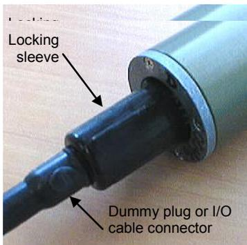
Verify that a cable or dummy plug is installed for each connector on the system before deployment.
