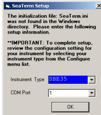
Select the instrument type (*SBE 35*) and the computer COM port for communication with the SBE 35RT. Click OK.
