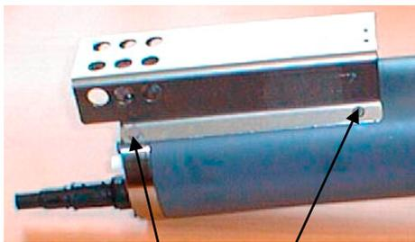
Do not remove socket head screw attaching guard to sensor end cap (2 places)
