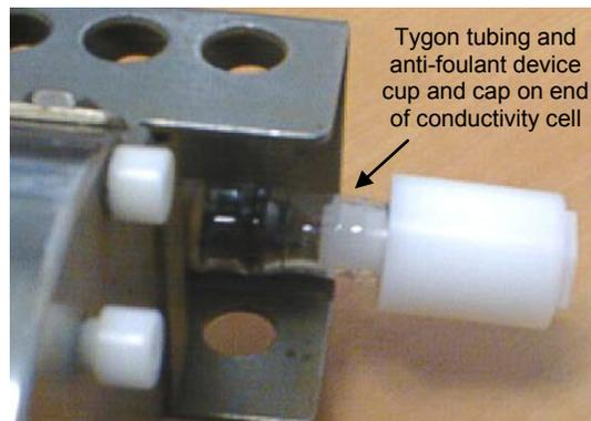
Tygon tubing and anti-foulant device cup and cap on end of conductivity cell
