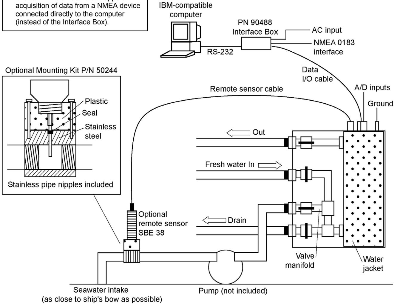
Valves are shown in normal operating position. Valves are open when handle is horizontal, closed when handle is vertical.
