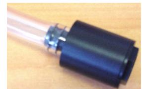
Alternate detail of Tygon tubing and anti-foulant device cup and cap – Sea-Bird began using black anti-foulant device cup and cap instead of white in 2008
