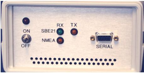
1. Connect *Serial* on the Interface Box to the computer using the DB-9S to DB-9P cable.
