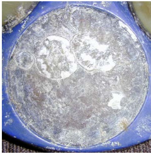
Figure 7. Barnacle Damage to Urethane Face
