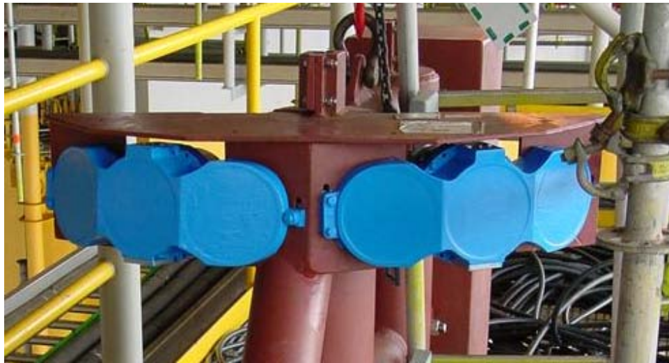
Figure 18. Antifouling Paint Applied on two H-ADCPs
