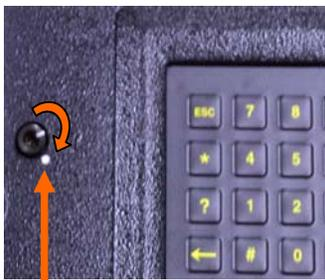
Newer 10-AU's are marked for the maximum clockwise turn rotation with a white dot. Do not turn the locking screw past this location.
