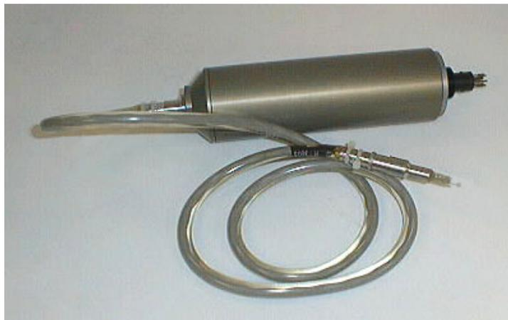
The sensing element is a remote-cabled, probe-mounted thermistor (Thermometrics type FP07). The sensor probe is a small, stainless steel assembly that may be mounted at distances up to 3 meters (9.8 ft) from the sensor electronics housing. This arrangement minimizes the effect of the instrument housing and its wake on the data. The thermistor body is O-ring sealed into the sensor assembly to ensure pressure integrity.
