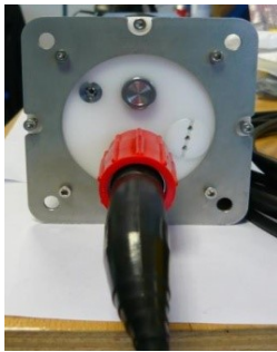
Connect SYLence recorder to Ethernet cable
