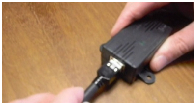
Connect cable to any computer Ethernet input
