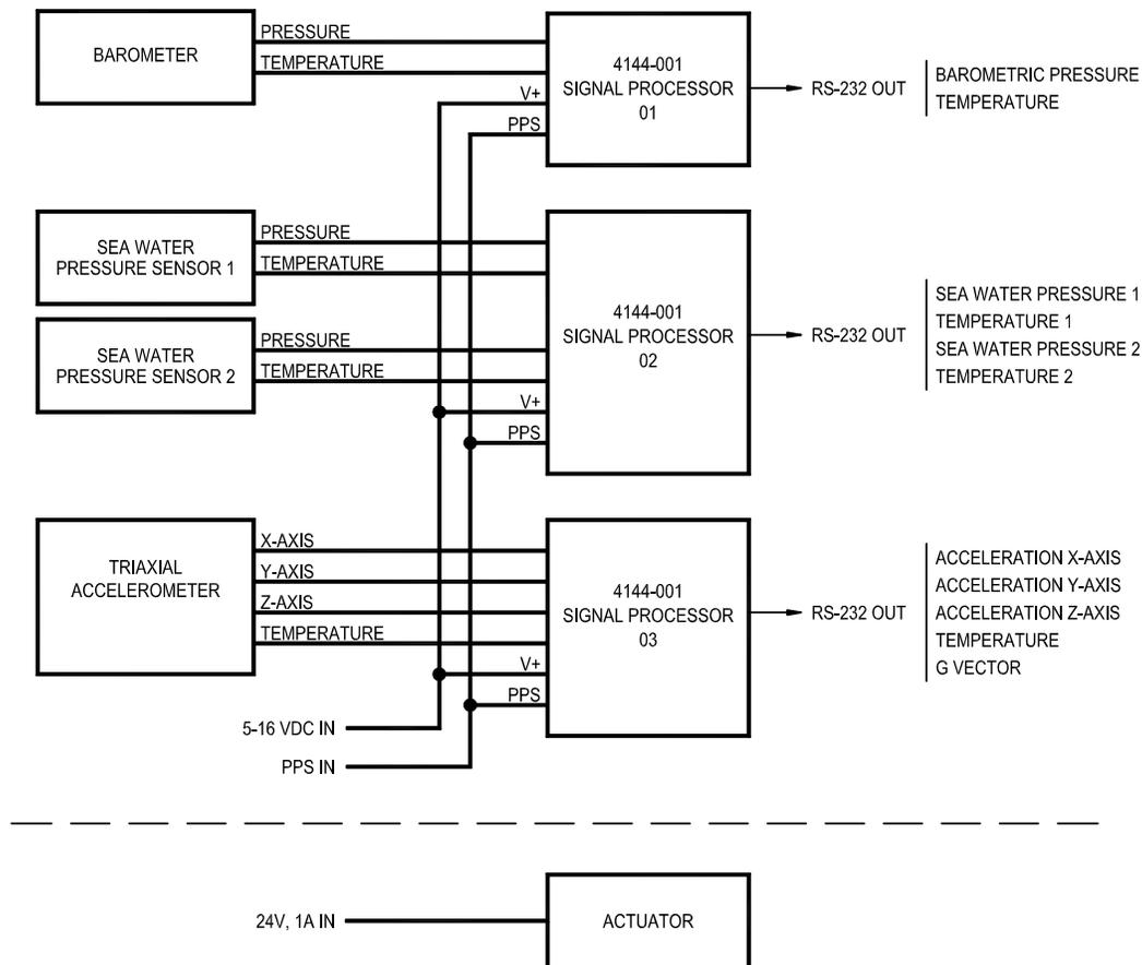
The GODS module contains (2) absolute pressure gauges with available ranges of 1400, 2000, 3000, 4000, and 7000 meters plus (1) Triaxial Accelerometer with an internal alignment matrix, plus (1) Digiquartz<sup>®</sup> Barometer, plus (3) Nano-resolution processing electronics. The pressure connection lines are vacuum oil-filled to (1) Swagelok 3-way ball valve that switches between seawater pressures, (A), and an interior oil reservoir, (0).
