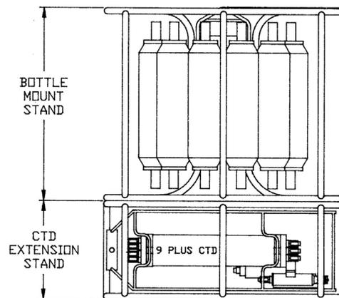
Note: Bottle mount stand height and diameter and CTD extension stand height varies, depending on number and size of bottles. See the SBE 32 specification sheet or manual for details.
