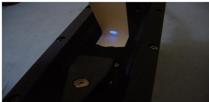
If there is no light from the sensor, check the power supply. If there is still no light, contact WET Labs Support.
