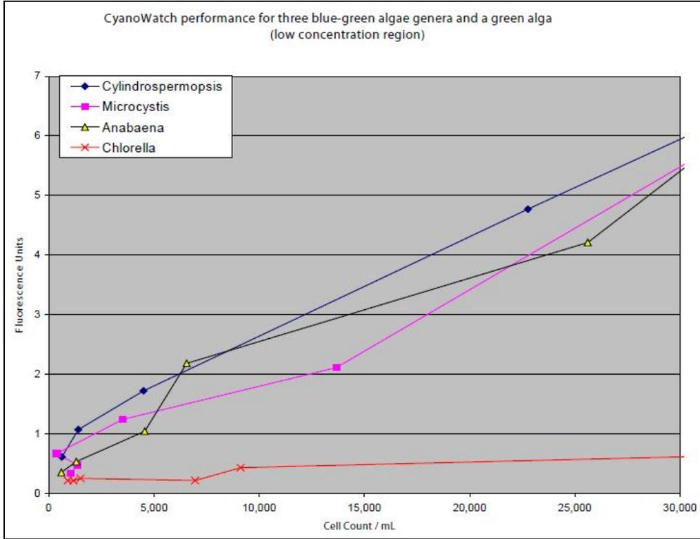
Figure 4 shows data collected from the Beta testing of a CyanoWatch on-line phycocyanin instrument. Three cultures of phycocyanin containing cyanobacteria were tested and one species of green algae as a control. The data indicates that the instrument detected all three cyanobacteria cultures at low concentrations while the green algae was not detected.
