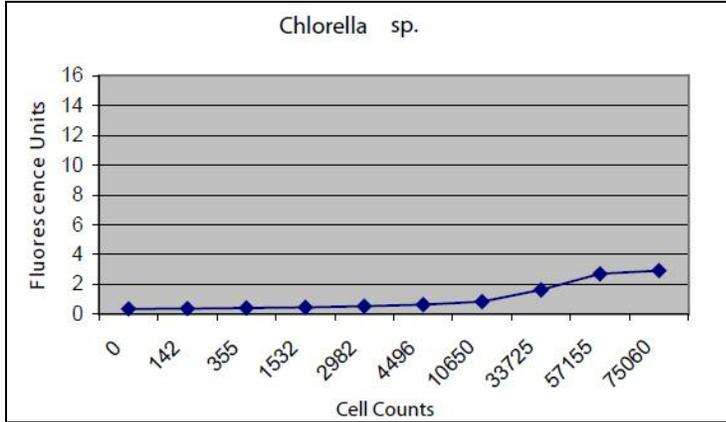
**Figure 9:** *Chlorella* sp. (a green alga containing no phycobilin pigments) sensitivity of the SCUFA-fluorometer with phycocyanin optics. The graph indicates that algal groups not containing phycocyanin do not interfere with the fluorescence readings.
