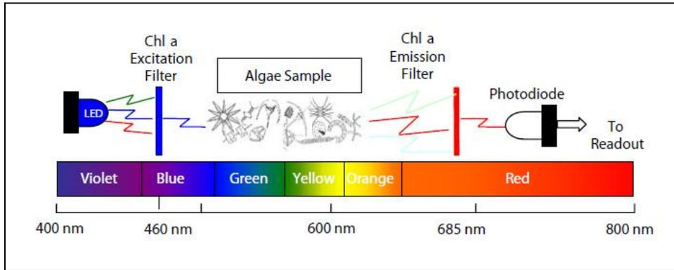
Figure 1: Fluorometer configuration for detection of chlorophyll /
