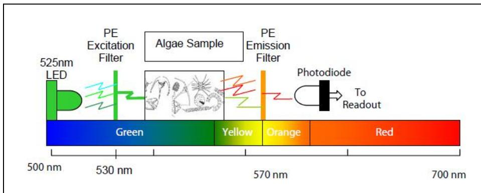
Figure 3: Fluorometer configuration for detection of phycoerythrin
