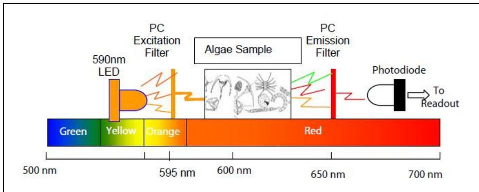
Figure 2: Fluorometer configuration for detection of phycocyanin
