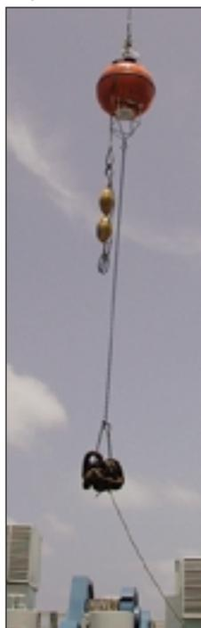
The upward looking, real-time current measuring system with anchor weight and instrumented buoy.
