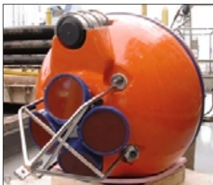
The one-metre diameter sphere with the embedded RDI ADCP and (at top) the Linkquest acoustic modem
