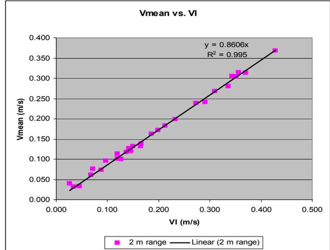
Figure 2 Measured mean velocity vs. Index-velocity: all data
