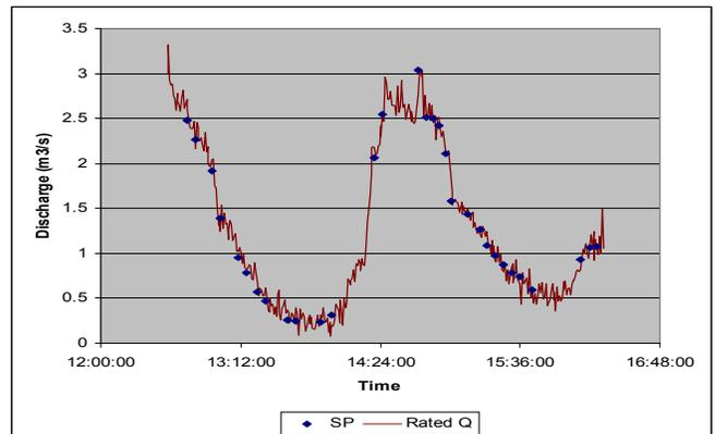
Figure 3 Time series of rated discharges and StreamPro measured discharges on December 9, 2003.
