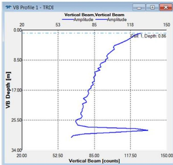
**Vertical beam(600kHz, 0.5 m cell size)**
