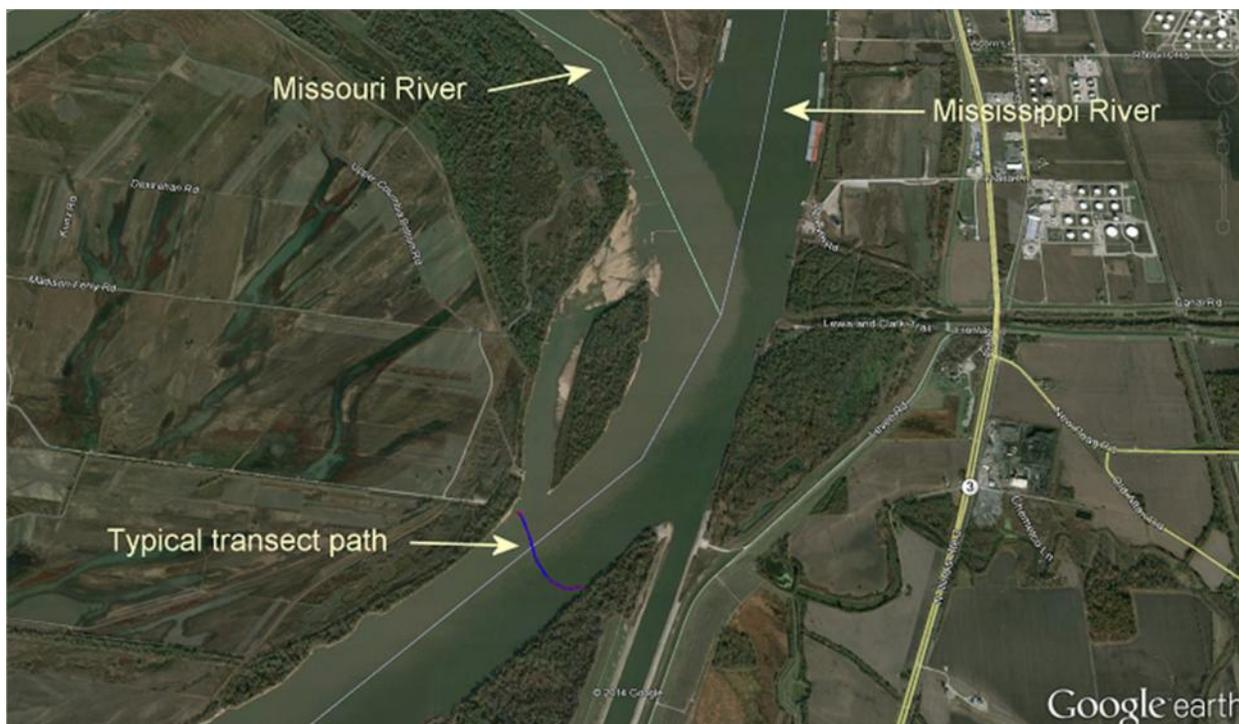
Figure 5. Ship track for measurements at the confluence of the Mississippi and Missouri Rivers
