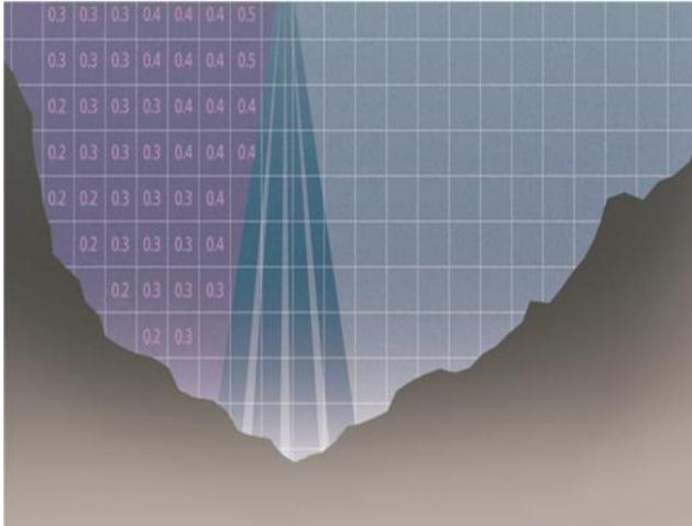
Figure 3. River section showing ADCP measurement grid
