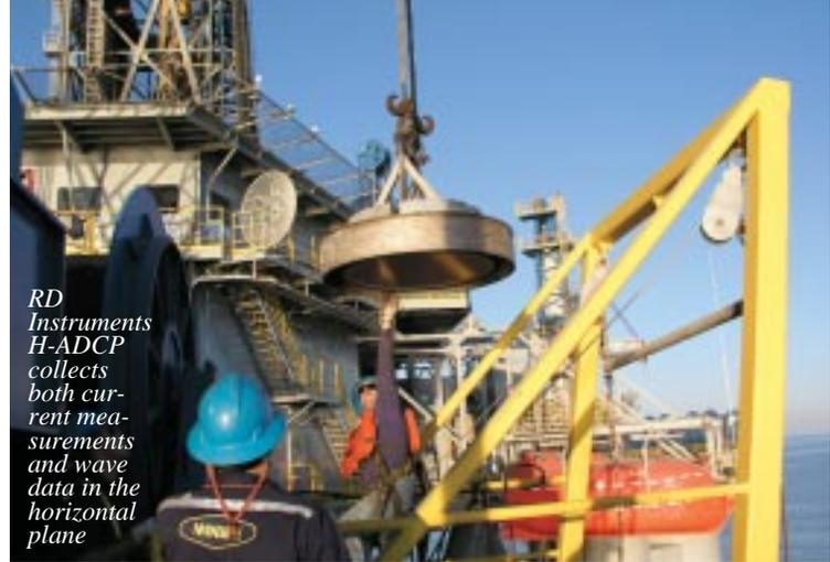
*RD Instruments H-ADCP collects both current measurements and wave data in the horizontal plane*
