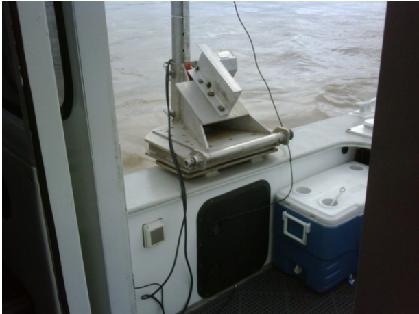
Figure 1: Mounting pole for the RiverRay or Rio Grande ADCP on the survey boat
