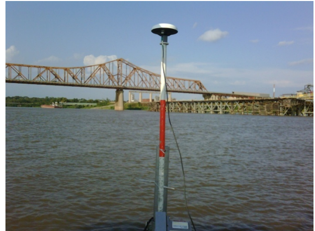
Figure 3: GPS antenna on the top end of the mounting pole
