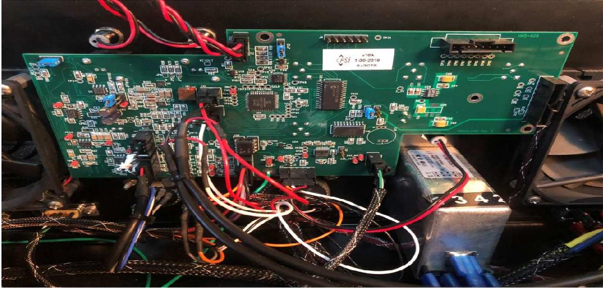
Disconnect the single green ground wire from the receiver board at the terminal lug behind the transformer. Make sure to note this location correctly for re-assembly.
