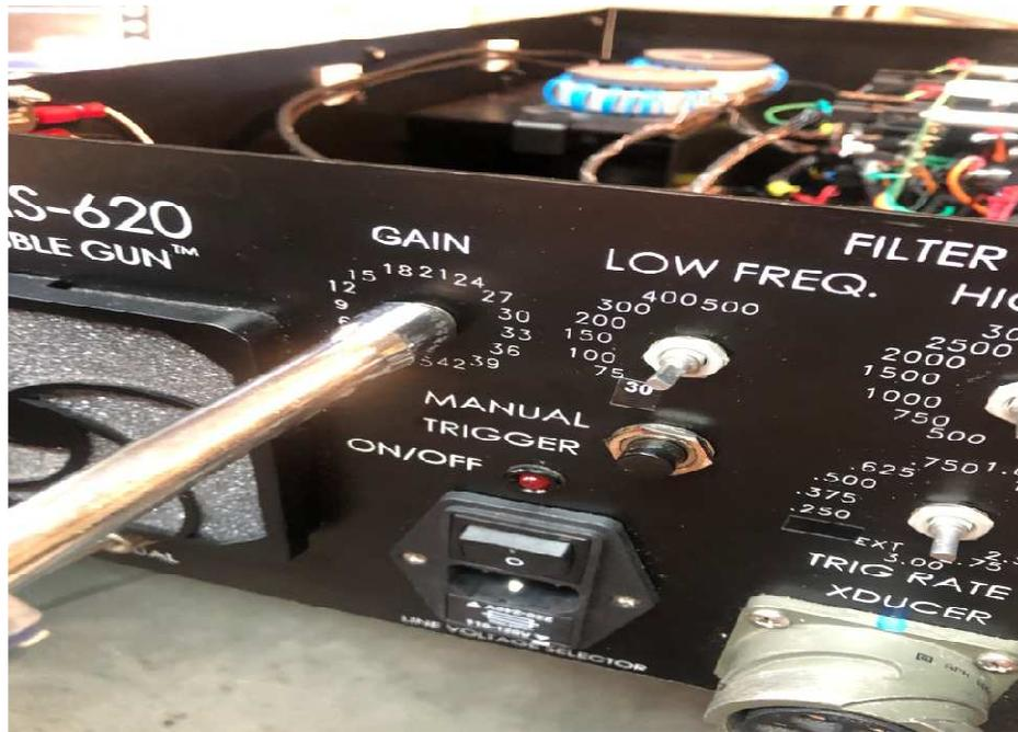
Remove the nuts and lockwashers from the (4) rotary switches and put the hardware in a safe place for re-assembly.
