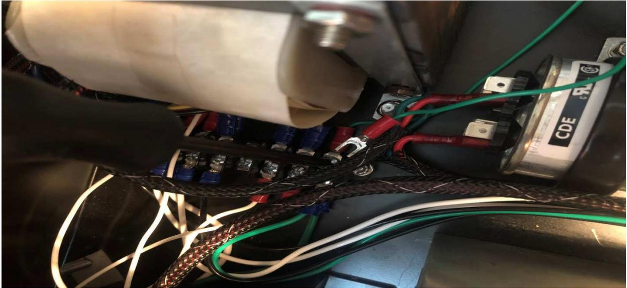
Remove terminal from lug and note location for re-assembly.
