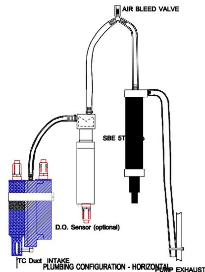
Figure 4 shows the horizontal configuration (CTD lying on its side), with the pump is mounted with its electrical connector toward the top end cap of the CTD. Tubing leads from the conductivity cell, (through the oxygen sensor plenum if an optional D.O. sensor has been installed) to the intake of the pump. The pump exhaust port is oriented so it points upward allowing air to escape as the CTD is submerged.
