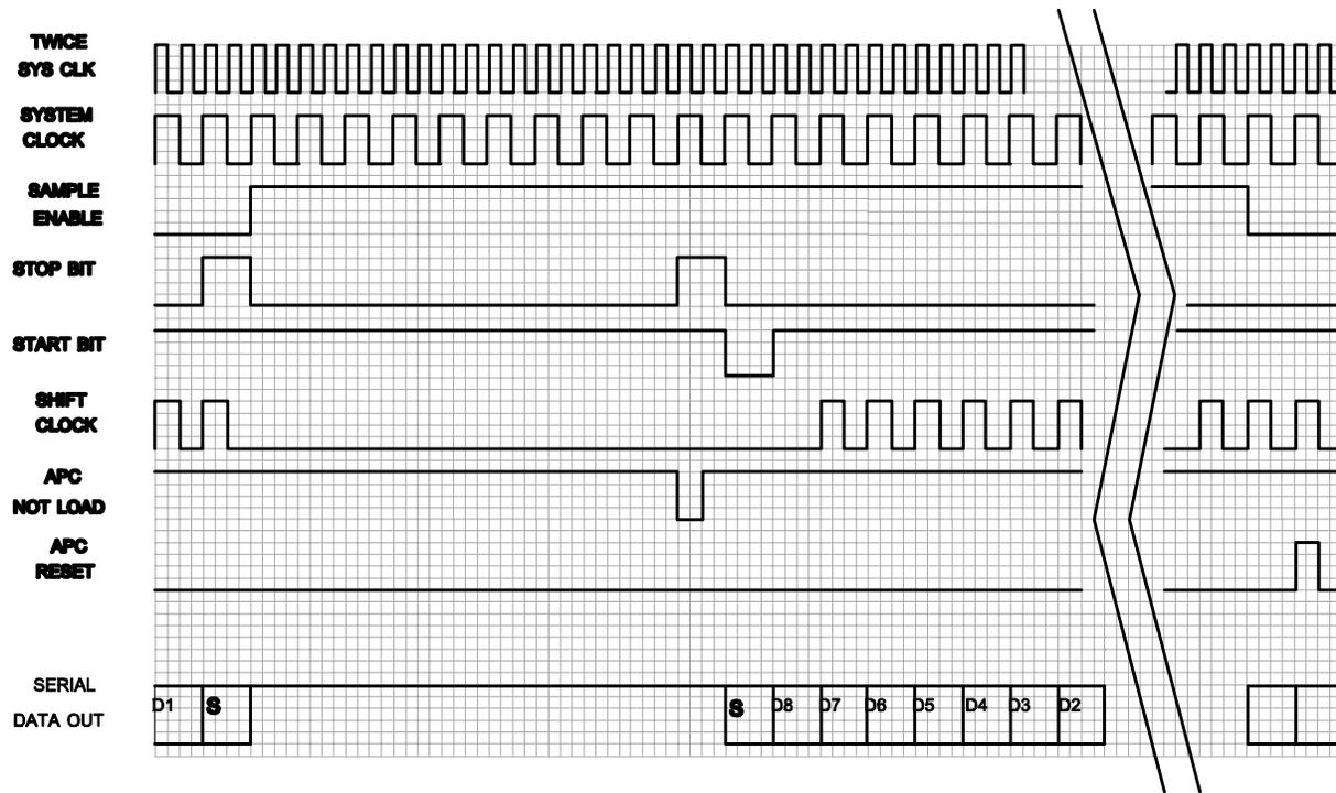
NOTE: APC not load ensures that the counting cycle ends in case of zero count. APC reset occurs after the falling edge of sample enable.
