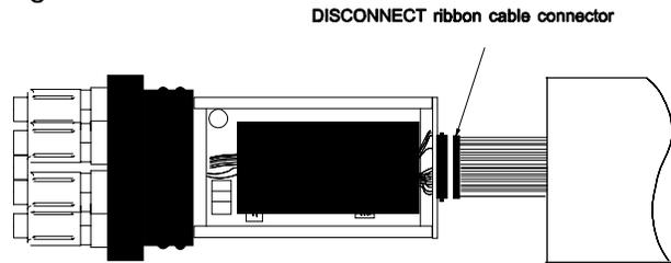
4) Unbolt the bottom end cap from the housing. Use the "jacking screws" to unseat the end cap (Figure 11). The card file will come out with the end cap, enabling you to work on the electronics.
