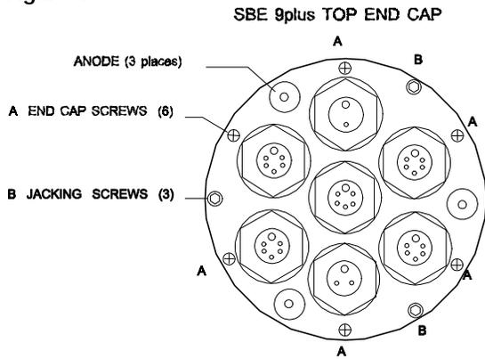
2) Remove the 6 screws which secure the top end cap to the pressure housing. Remove the top end cap using the white plastic "jacking screws" provided. (Figure 9)
