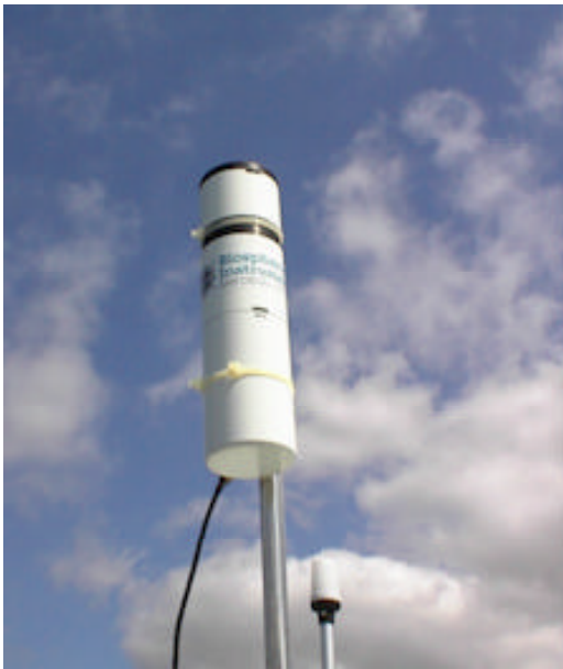
The PUV-2510 may be used as a surface reference for the PUV-2500 or as a stand-alone UV-PAR surface instrument
