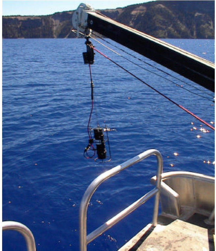
The PUV-2500 may be deployed by hand or overhead crane.
