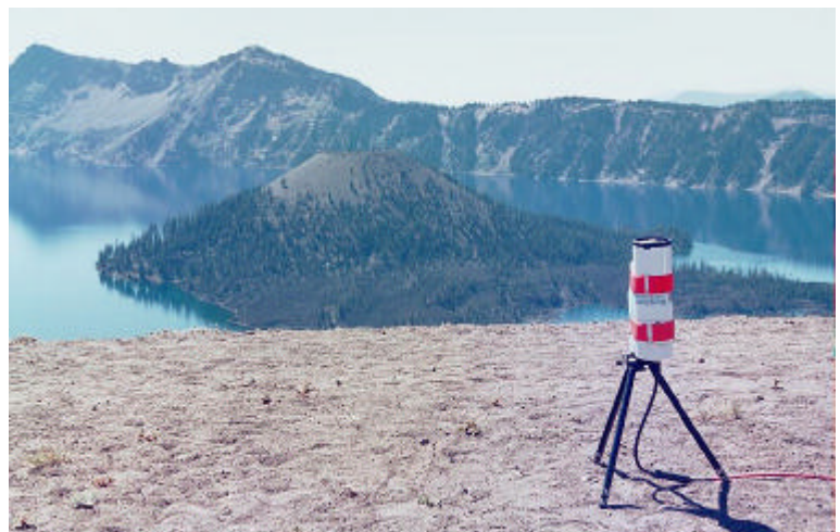
The PUV-2510 may be used as a surface reference for the PUV-2500 or as a stand-alone UV-PAR surface instrument
