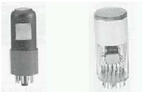
**Figure 4. Side-on PMT and End-on PMT**
