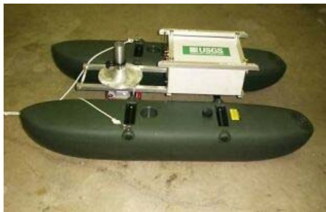
Hobie Floatcat modified for use with Rio Grande ADCP.
