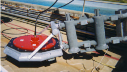
Fig. 14: deployment of the PA-38 ADCP that was used to collect the data presented in this paper, Shell E & P Technology Company.
