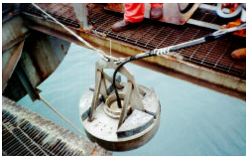
Fig. 2 Deployment of a PA-38 ADCP on an Oil Rig
