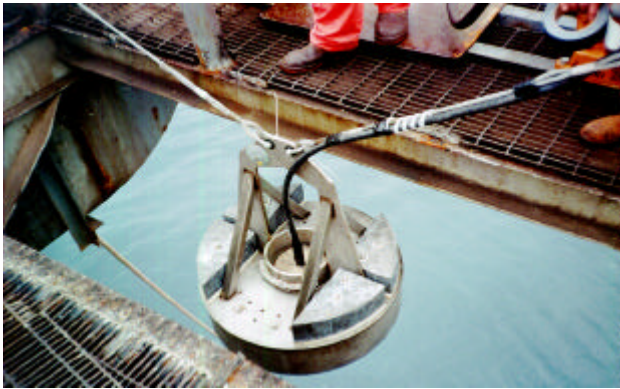
Fig. 1.--PA-38 ADCP deployment frame for suspension off a Drilling rig.
