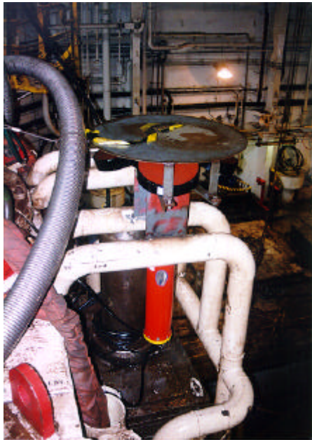
Fig. 2.--BOP mounted 75 kHz ADCP, transducers are just visible below protective steel cover, which is removed prior to deployment.
