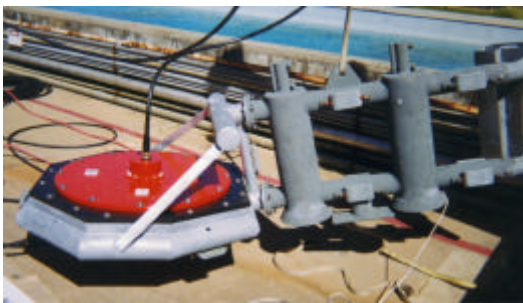
Fig. 9.—Deployment frame of the PA-38 ADCP that was used to collect some of the data presented in this paper.
