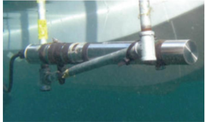
SUNA deployed for longitudinal profiling.
