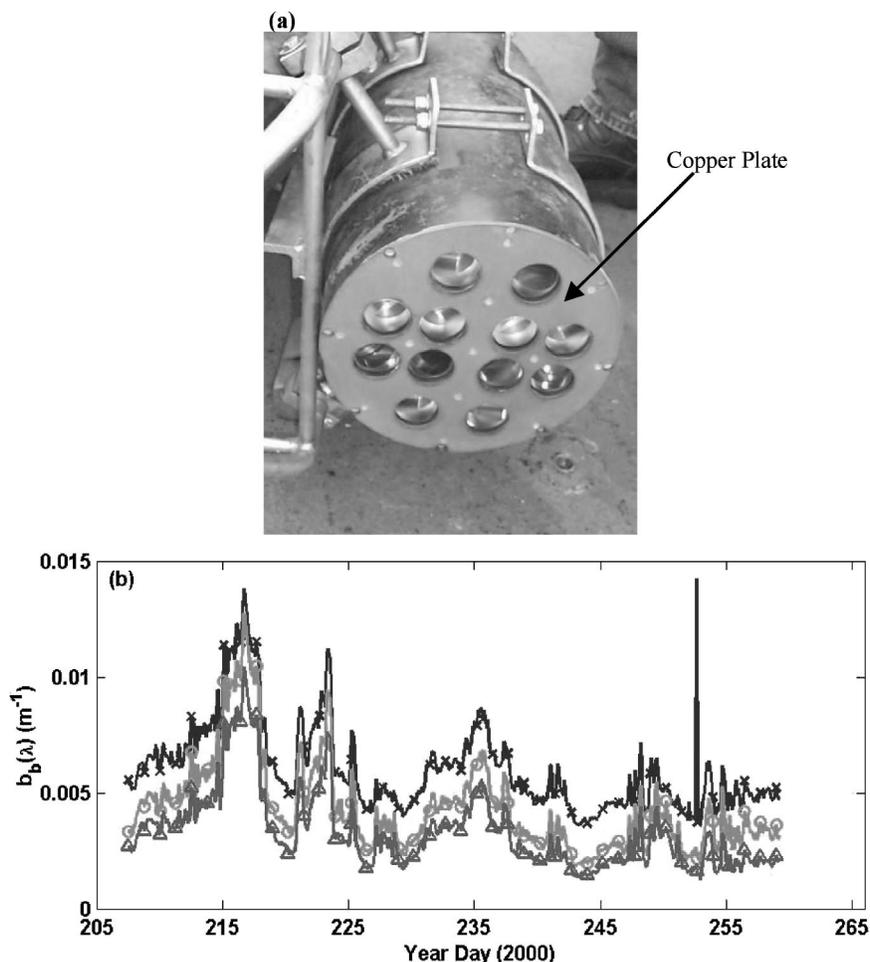
FIG. 1. (a) Photograph of the cupronickel endplate mounted on a HOBI Labs Hydroscat-6 backscattering instrument and (b) a 60-day, level 0 (nonbiofouled) time series of backscattering data at three wavelengths measured by the copper-plated Hydroscat-6 (xs, 442 nm; circles, 510 nm; triangles, 620 nm). The instrument was deployed at 5 m in 25-m water depth off of the coast of NJ during HyCODE.
