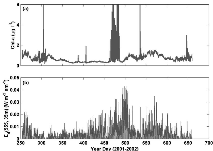
FIG. 5. A 410-day time series of level 0 (nonbiofouled) (a) 6-h-averaged chlorophyll-*a* concentration derived from a copper-shuttered ECO fluorometer and (b) downwelling irradiance at 555 nm measured with a copper-shuttered radiometer. Both instruments were deployed at 35 m in the Japan Sea from Sep 2001 to Oct 2002.
