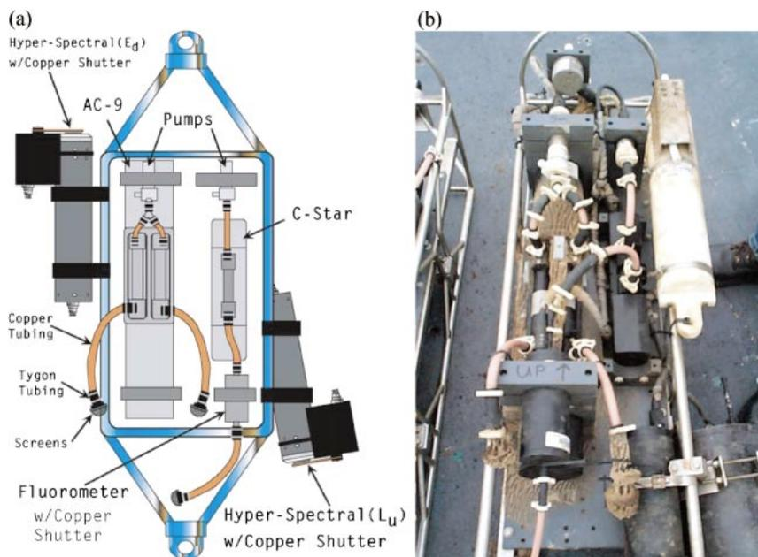
FIG. 3. (a) Schematic diagram of a biooptical system package illustrating the copper tubing used for the flowthrough optical instruments and copper shutters and (b) photograph of a biooptical system recovered after a 2-month deployment. Note the growth of macroalgae on the components of the instrument package while the copper tubing remained free of biofouling. Also note that (a) and (b) are not the same instrument package.
