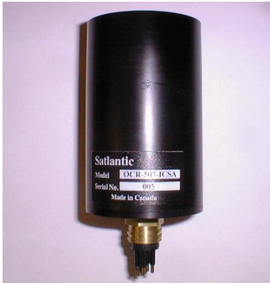
*Figure 1: OCR-507 (in air) - Irradiance Configuration*
