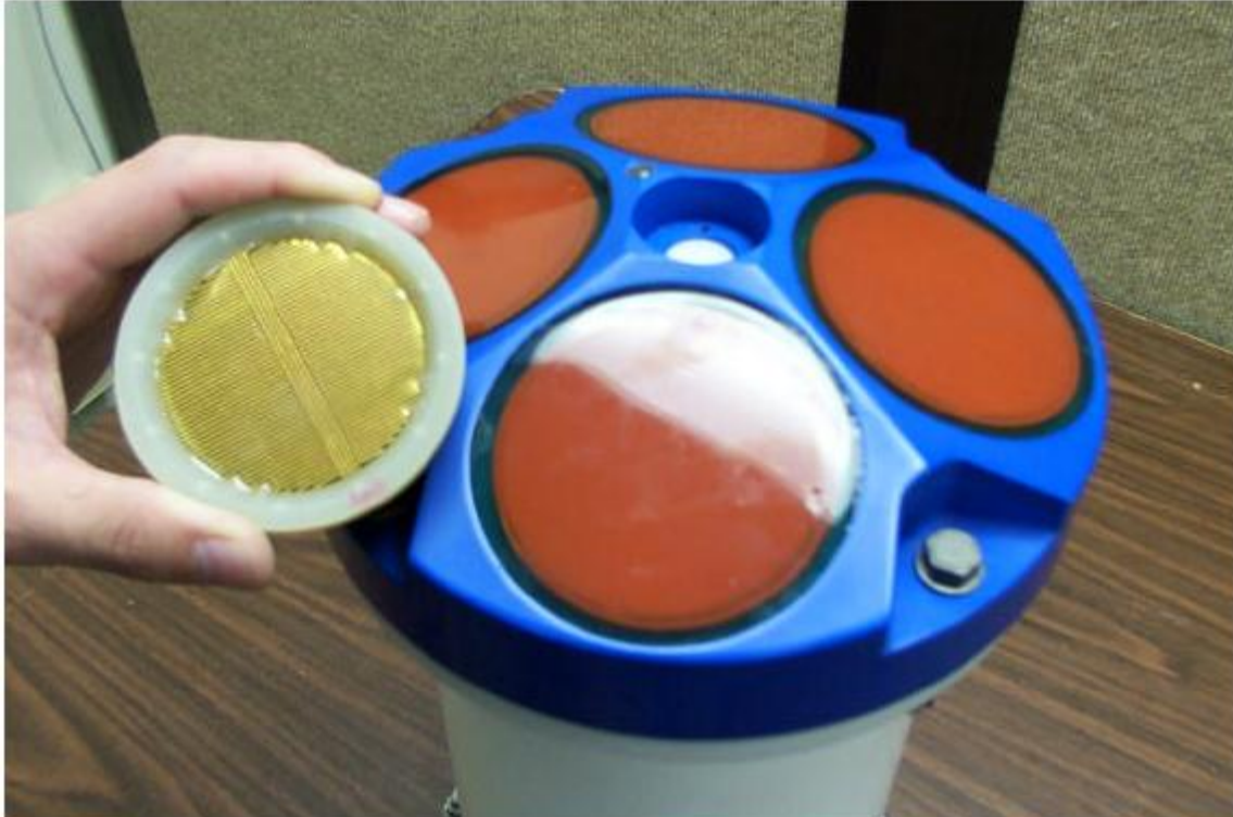
Figure 31. Comparison of a 600kHz developmental phased array transducer with a standard four piston 600kHz WorkHorse transducer.
