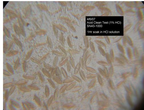
Fig. 3 100X magnification of an SBE 43 DO sensor membrane covered with biological growth. Taxonomic analysis revealed diatoms on the membrane. This sensor was deployed for nine months with no servicing or maintenance in Cockburn Sound, Perth, Western Australia.
