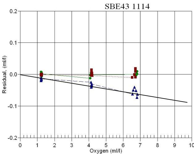
Fig. 2 Calibration results of oxygen concentration (x-axis) and residual concentrations (y-axis) between replicate Winkler water samples and SBE 43 sensor values in a temperature-controlled bath. Dots specify the original calibration, triangles show post-calibration results (prior to cleaning), and squares denote the final calibration results (after cleaning).
