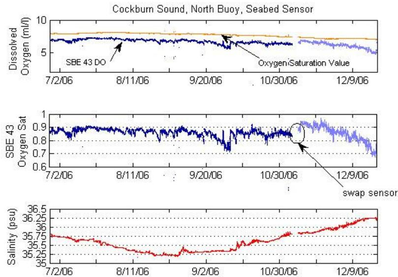
Fig. 1 Near-bed oxygen and salinity at the North buoy in Cockburn Sound for period June 26 – December 22, 2006. SBE 43 sensor 0986 was recovered on November 9, 2006, cleaned and redeployed on a different mooring and is still in the field. Top Panel: Time series of sea-bed measured dissolved oxygen (blue Jun-Nov; purple Nov-Dec) and theoretical saturation concentration (gold); Middle Panel: ratio of SBE 43 measured oxygen to oxygen saturation; Bottom Panel: sea-bed salinity.
