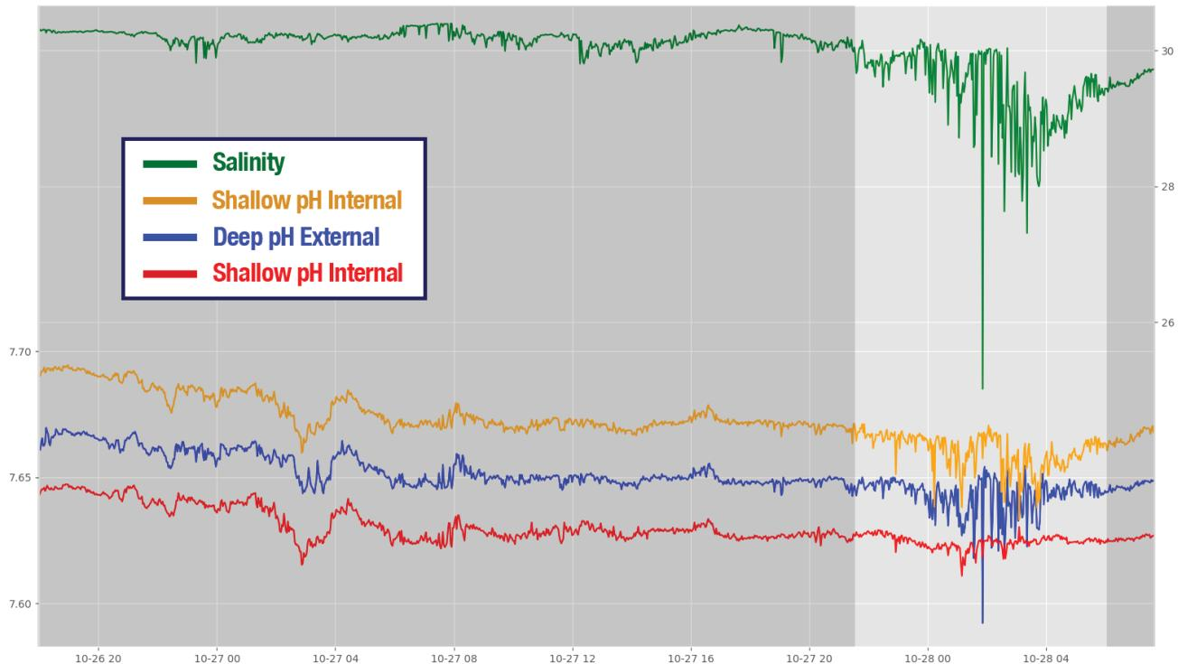
The highlighted section shows a 4-hour period of high rainfall, where salinity varied significantly. **The resulting pH data during this period from the Deep SeapHOx V2 (blue) and pH External from the Shallow SeapHOx V2 (orange) shows significantly more noise than the pH Internal values from the Shallow SeapHOx V2 (red).** Other deployments have shown that pH External can have a slower response to changing pH after large salinity swings. **The magnitude of error is typically within 0.05 pH.**
