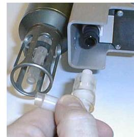
4. Retighten the temperature sensor guard by hand.
